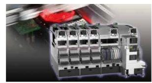
The operator just pushes the START button after exchanging the head. The machine automatically performs calibration for the head and restarts production.
