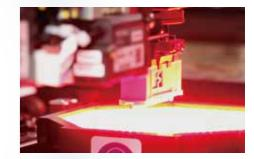
Large connectors can be reliably inserted at one time
