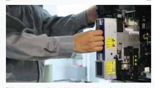
Fuii's original compact lightweight heads that can be easily exchanged without using tools. Operators on-site can perform maintenance and handle troubles.
