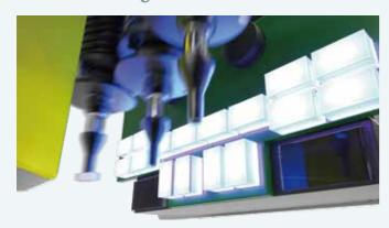
Checks tombstoned parts, missing parts, and up-side down parts IPS can cater to a wide range of checks, from part pickup stance to parts remaining on nozzles, as well as upside-down checks for minimold parts. Placement defects caused by packaging, nozzles, and parts can be prevented.
