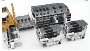
Increase the capability in minimum units of 645 mm and supports the latest placing processes by adding various units. Costs can be greatly reduced because adding new lines is not required.
