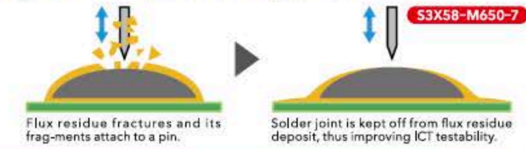
Figure 1. Example of ICT inspection failure
