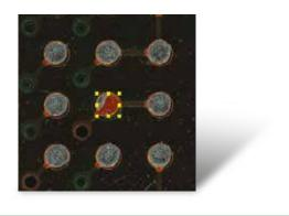
Precise height measurement based on Phase Measurement Profilometry (PMP). Bi-directional phase shifting projection system ensures accurate and noise resistant measurement of the paste height and volume.
