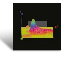
Innovative, real-time automatic warpage compensation and measurement floor recognition method. The system identifies the pads as a zero level for the paste height measurement for each board and FOV. Such a capability completely eliminates the influence of PCB warpage on the inspection result. The process is completely automatic and user-independent, no bare board or any special procedures are required.
